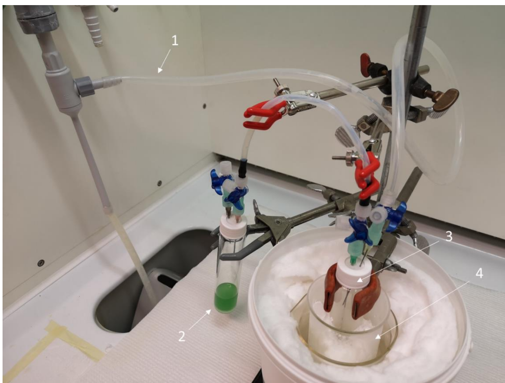
Fig. S1 Customized trapping system used to capture isoprene from the culture tubes (1 - vacuum line; 2 - culture tube; 3 - collector tube; 4 - acetonitrile / dry ice slurry at -40 °C).
