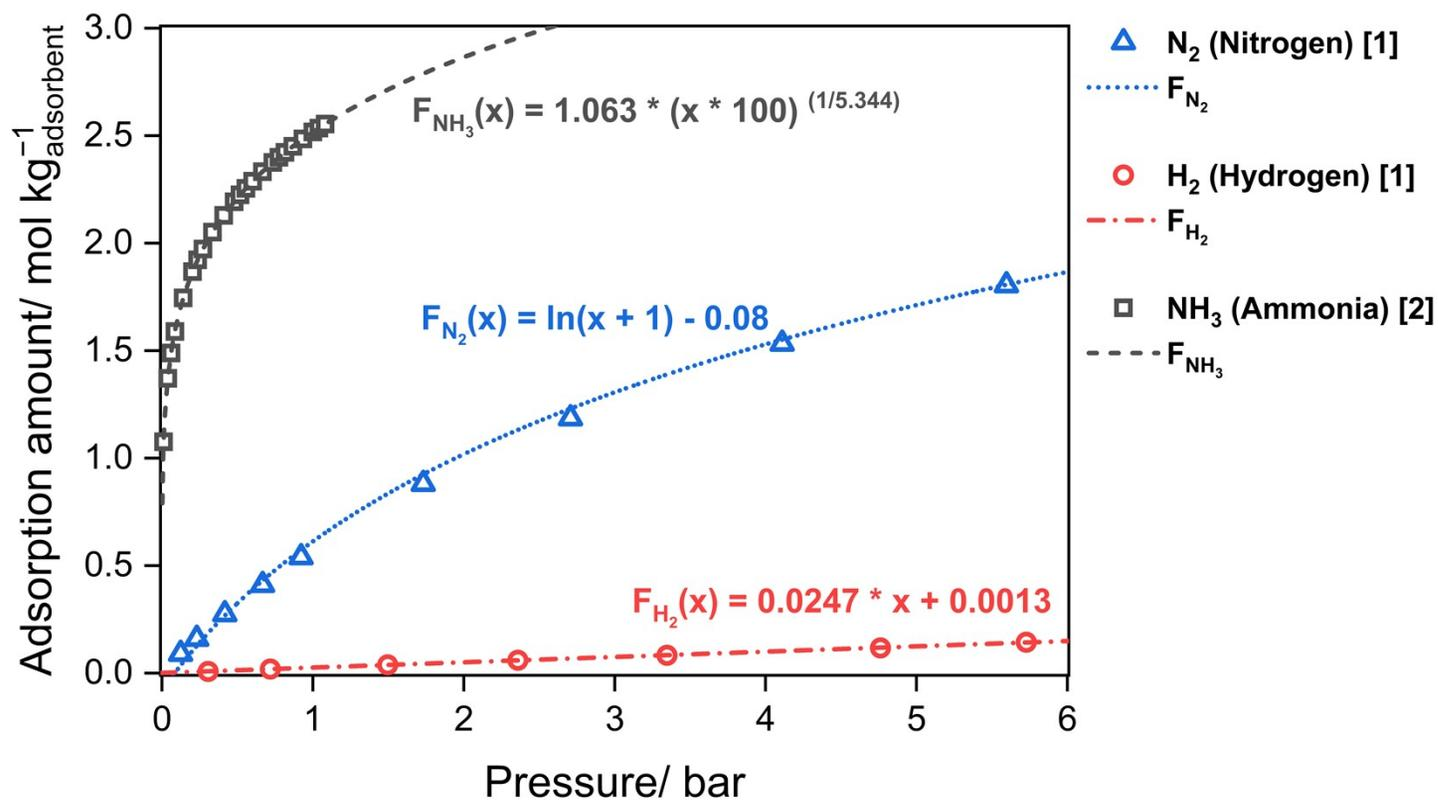
Fig. S2 Adsorption isotherms of nitrogen and hydrogen on 5A zeolite and ammonia on alumina.<sup>1,2</sup>
