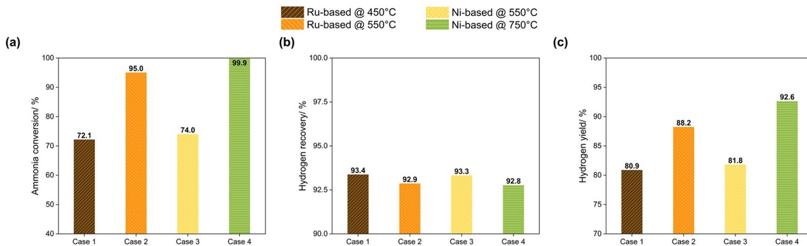
**Fig. S5** Technical performance of the cases in this study in terms of (a) ammonia conversion in a reformer, (b) hydrogen recovery in pressure swing adsorption, and (c) hydrogen yield in the overall system.
