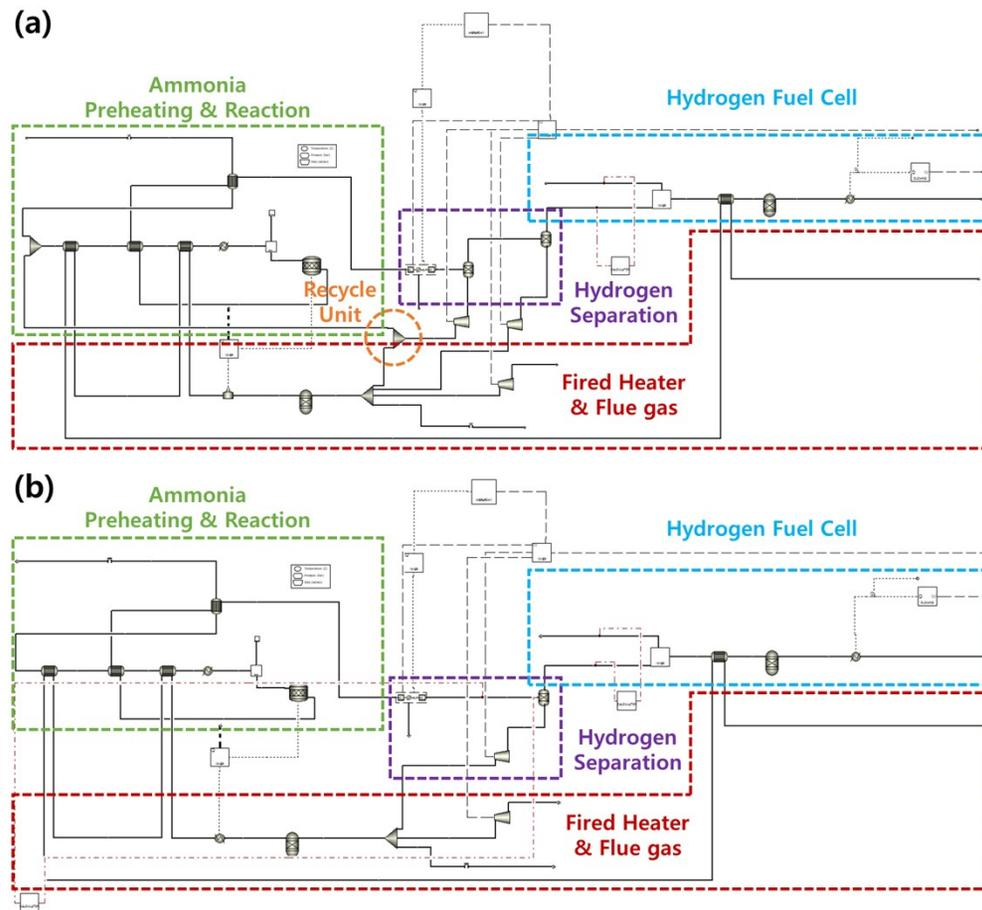
**Fig. S1** Aspen flow sheet of the proposed power generation system based on ammonia decomposition and hydrogen fuel cell (a) Cases 1 and 3, which have a recycle stream due to low conversion of ammonia and (b) Cases 2 and 4, which present sufficiently high conversion of ammonia.
