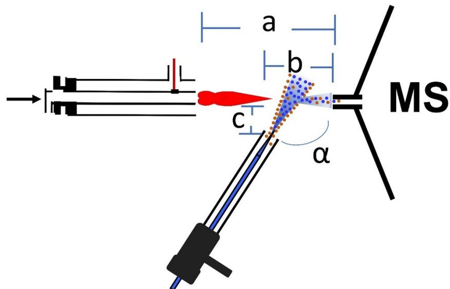
**Figure S2** Schematic illustration of the setup of sample introduction system. The distance **a** between the MPT tip and the ion entrance of the LTQ instrument was 2.0 cm; the distance **b** between the tips of MPT plasma and MS inlet was 1.0 cm. The distance **c** between sample introduction device and MPT plasma was 0.5 cm. The angle  **$\alpha$**  formed between sample introduction device and the axis of the sampling cone was 120°.
