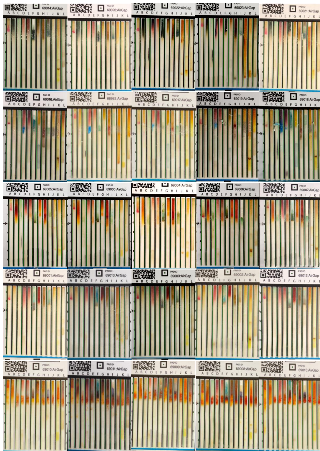
Figure S6. Air-gap 12-lane pharmaceutical-screening PAD images. Top row: amoxicillin, 2 nd row: ciprofloxacin, 3 rd row: isoniazid, 4 th row: pyrazinamide, bottom row: rifampicin.
