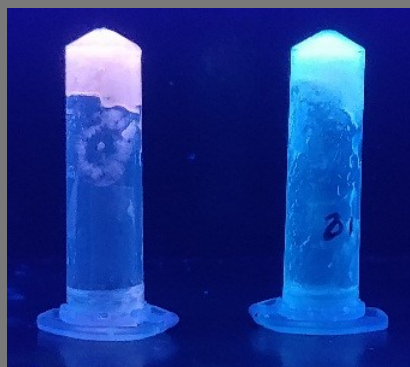
Figure S6. Photographs of Eu(III) and Tb(III) gel under UV light. (Vial inversion test for confirming gel formation).
