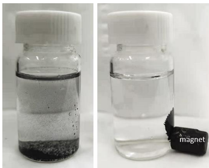
Figure S3. Schematic diagram of Co-400 catalyst dispersed in aqueous solution (left); Schematic diagram of Co-400 catalyst dispersed in aqueous solution after adsorption with magnet (right)
