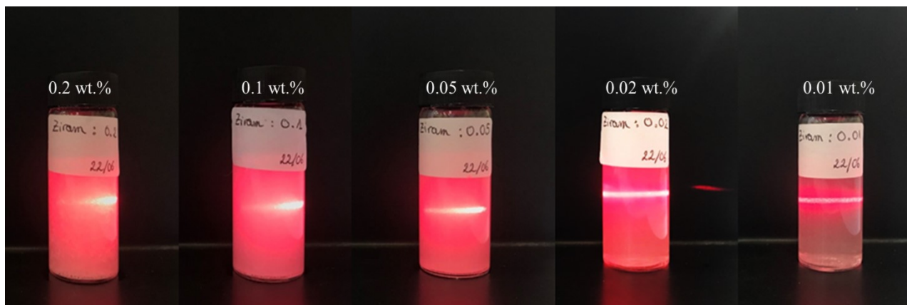
Figure S1. Ziram solubility test of: 0.2 wt. %, 0.1 wt.%, 0.05 wt. %, 0.02 wt.%, and 0.01 wt.% Ziram solutions at pH 8.
