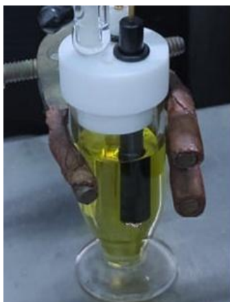
Fig. S24 Photograph of the customized, one-compartment, three-neck cell with a glassy carbon working electrode. \text{H}_2 gas bubbles are appeared on the surface of the working electrode.
