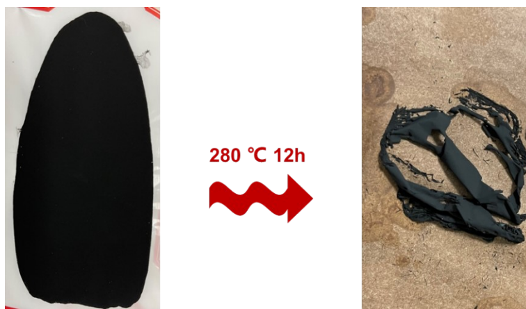
Figure S6 The OV-BaTiO 3 @RGO@PP separator c after heat treatment.
