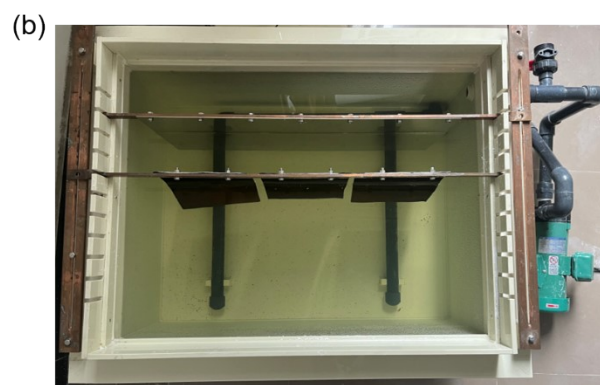
Fig. 18. The physical diagram of the reactor: (a) side view and (b) vertical view.
