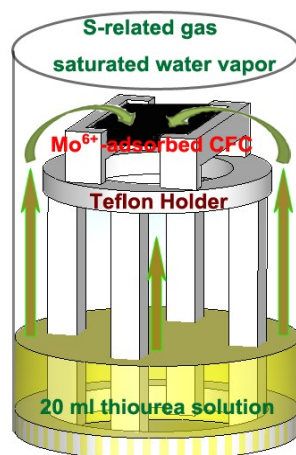
Fig. S2 Experimental set up of vapor-phase hydrothermal (VPH) method used in this work.
