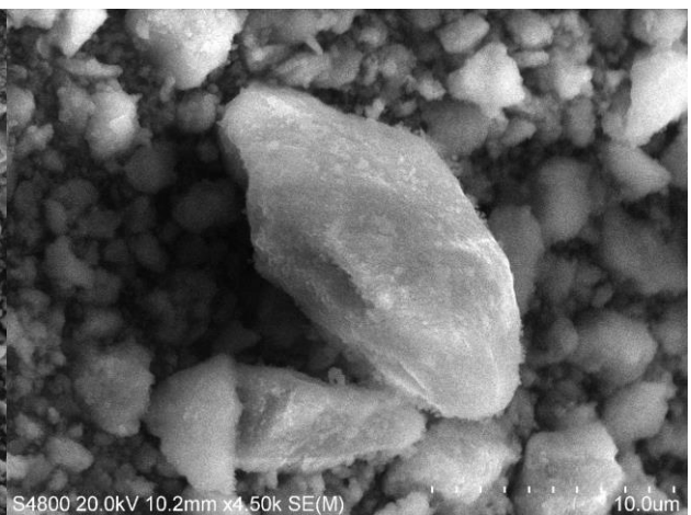
Figure S2. SEM image of (a)–(b) SG85 porous zirconia, (c)–(d) SG85-ATMP, (e)–(f) SG85-EDTMP, (g)–(h) SG85-DTPMP and (i)–(j) SG85-TTHMP.
