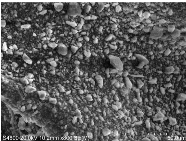
Figure S2. SEM image of (a)–(b) SG85 porous zirconia, (c)–(d) SG85-ATMP, (e)–(f) SG85-EDTMP, (g)–(h) SG85-DTPMP and (i)–(j) SG85-TTHMP.
