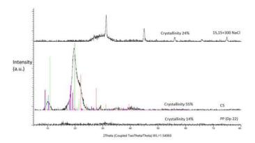
Figur S1. X-ray diffraction spectrum of PP, CS powder, and (15,15+300) beads
