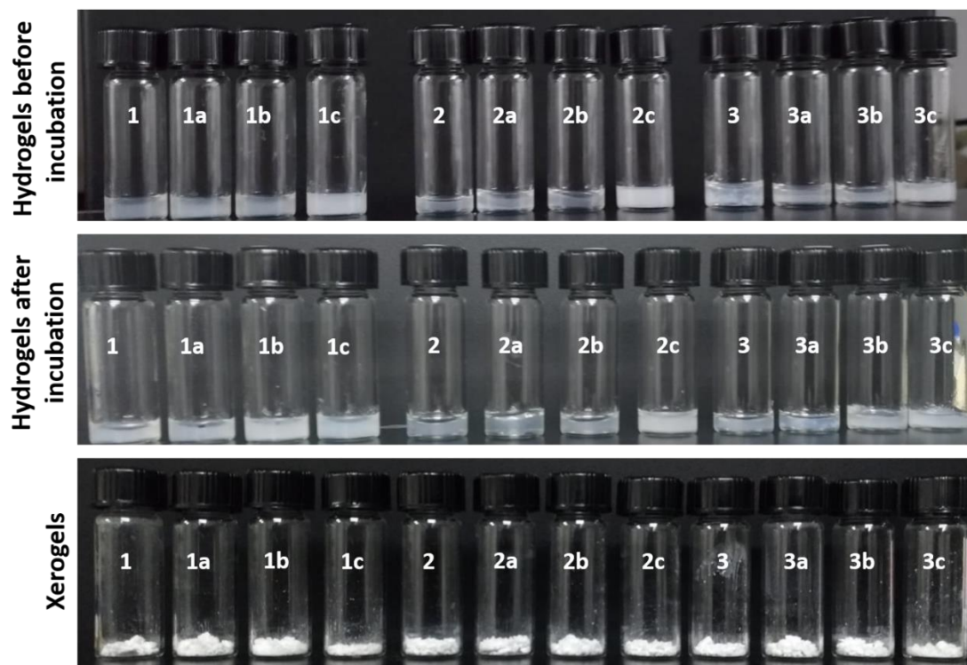
Fig.S16 Gel stability: Optical images of hydrogels before and after incubation with phosphate buffered saline (PBS) 7 days at 37 °C and their corresponding xerogels.
