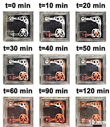
Fig. S4. Photographs showing the siphon effect of the liver-lung multi-organ-on-paper platform with three layers of printed structure at the 6 mm of height of the medium reservoir with 3 mm in diameter of the evaporation opening of volatilization chamber at different time points.
