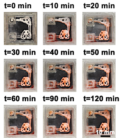
Fig. S5. Photographs showing the siphon effect of the liver-lung multi-organ-on-paper platform with three layers of printed structure at the 10 mm of height of the medium reservoir with 3 mm in diameter of the evaporation opening of volatilization chamber at different time points.
