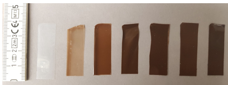
Figure S3. Composite films with different loading of IONPs. From left to right: 0, 0.3, 1.3, 2.6, 3.9, 5.1, 11.9 wt%.
