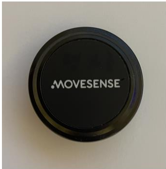
Fig. S10 Photographic images of the Movesense sensor (MODEL: OP174; diameter 36.6 mm & weight 9.4 g) (a) front and (b) back.
