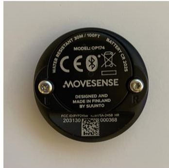
Fig. S10 Photographic images of the Movesense sensor (MODEL: OP174; diameter 36.6 mm & weight 9.4 g) (a) front and (b) back.
