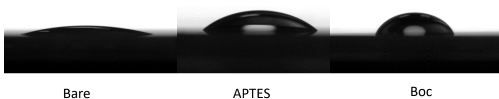
Figure SI- 8: water contact angle measures on glass samples (a) bare sample, (b) APTES functionalized, (c) boc functionalized glass.
