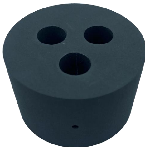
Figure S1. Photograph of one of the custom, cylindrical three-sample graphite dies used for spark plasma sintering (SPS, S-sintering) with a height of 30 mm, outer diameter of 60 mm, and inner diameter of 3x \varnothing 10 mm.
