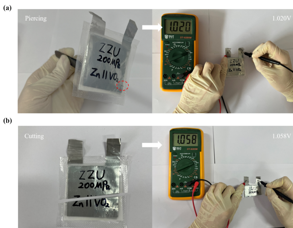
Figure S11 Piercing and cutting experiments
