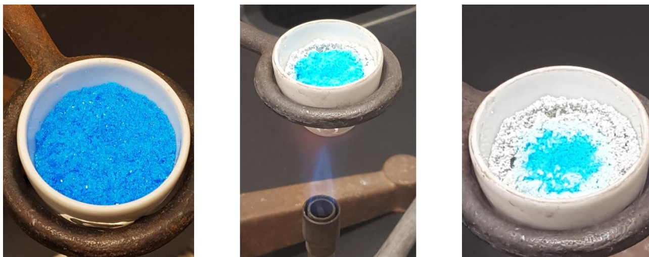
Figure S1. A popular demonstration of dehydration. The blue pentahydrate (at left) on heating with an open flame (center) visibly loses water as steam and the core shows progressively paler blue towards the edge (right), which is commonly described as the anhydrous sulfate.
