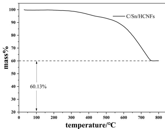
Fig. S1 The TG curves of C/Sn/HCNFs composite materials
