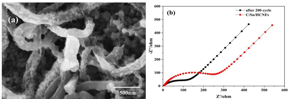
Fig S4(a) SEM image of C/Sn/HCNFs after 200 cycle charge and discharge, (b)EIS curves of C/Sn/HCNFs and after 200 cycles.
