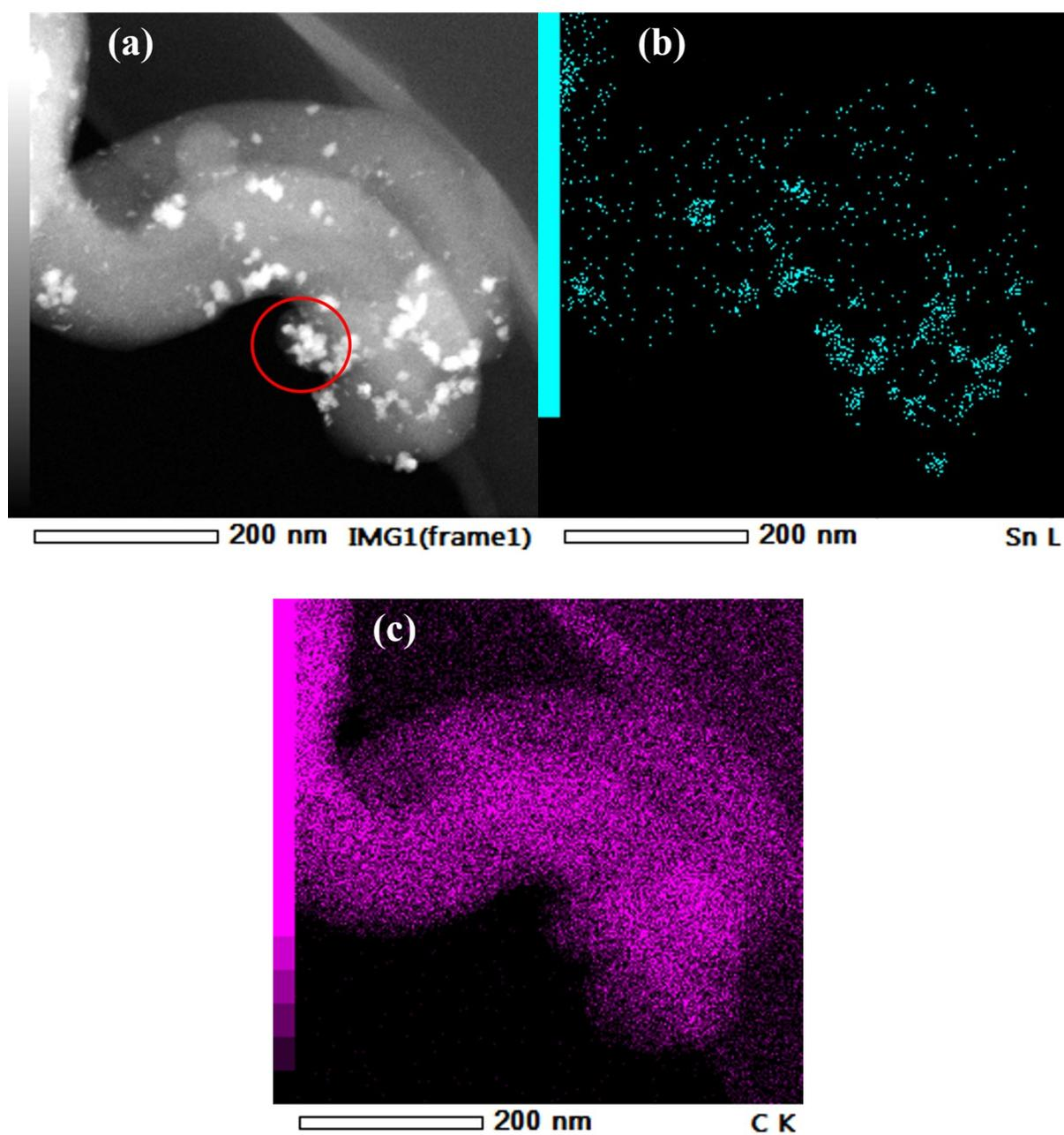
**Fig. S3** EDS elemental mapping of STEM image (a) C/Sn/HCNFs; (b)Sn element; (c)C element
