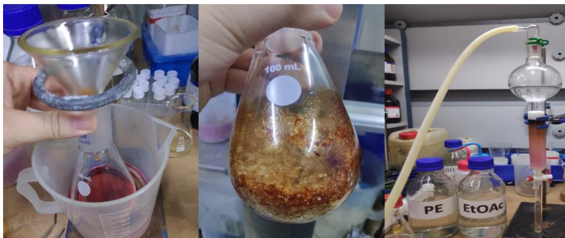
(Left) Filtered. (Center) The crude product; (Right) Purified by chromatography on silica gel (PE/EtOAc = 3:1).
