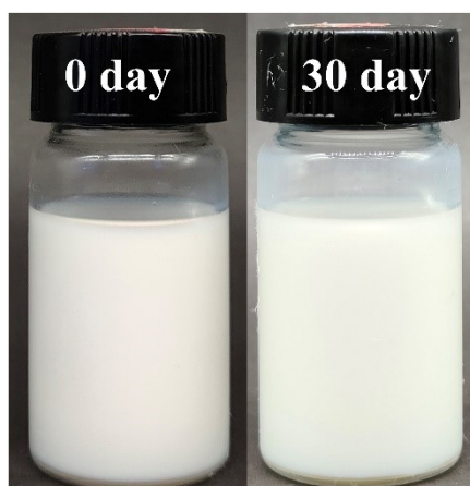
Fig. S9 The Polyacrylamide emulsion stabilized by 3 wt % DM-OA
