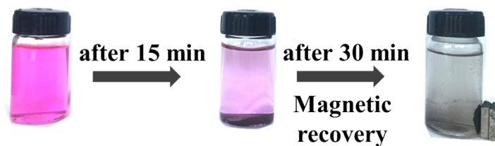
Figure S4 Degradation of RhB and recovery of micromotors by magnetic field.
