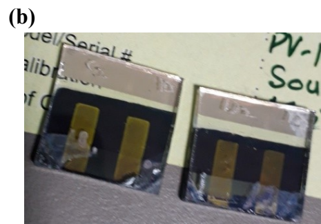
Figure S3. (a) Device demonstration by using P3HT and Spiro-OMeTAD as HTL in FTO/SnO 2 /MAPbI 3 /HTL/Ag (b) Silver electrode degradation and its corrosion on the devices where P3HT and spiro-OMeTAD are used as an HTL in the device of structure FTO/SnO 2 /MAPbI 3 /HTL/Ag.
