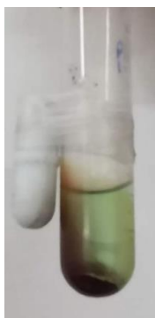
Figure S1. Washing solution from sample A0 processed at 140°C for 16 h.
