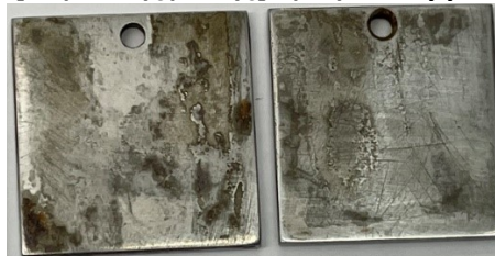
Figure S8: Visual comparisons pictures of few sample coupons after 7 days immersion in inhibitor solutions in NaCl 0.01M. (Left – Trial 1; right – Trial 2.)
