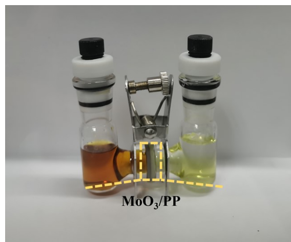
Fig. S4. Li 2 S 6 permeation experiment of H-shaped glass tubes with MoO 3 /PP.
