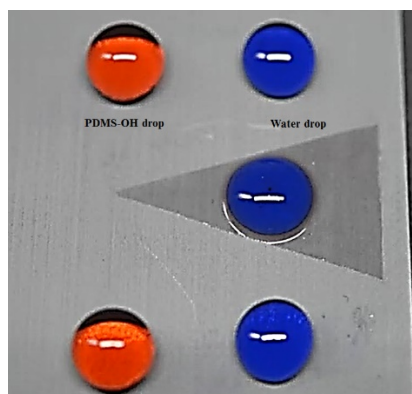
Fig. S2. Demonstration of hybrid superamphiphobic-slippery patterned surface. Water and PDMS-OH drops stood still on superamphiphobic surface, however, PDMS-OH drops spread on wedge-shaped superhydrophobic surface. Water was dyed in blue while PDMS-OH was dyed in red.
