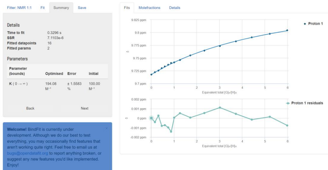
Fig. S1 The corresponding isotherm of macrocycle 1 with n Bu 4 NAcO based on a 1:1 model using the www.supramolecular.org web applet, giving K_a = 194 \text{ M}^{-1} . The monitored signal was corresponding to amide NH protons. The residual distribution was displayed below the binding isotherm.
