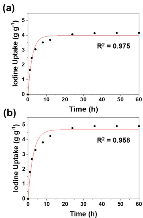
Fig. S8. The pseudo-first-order kinetic model of (a) NI-COF-1 and (b) NI-COF-2.
