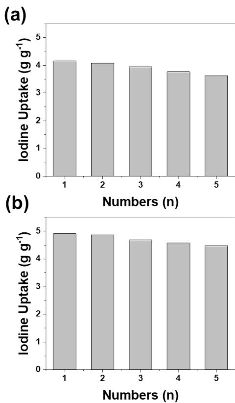
Fig. S12. Recycle performances of (a) NI-COF-1 and (b) NI-COF-2.
