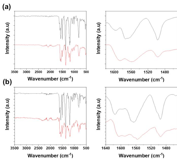
Fig. S10. FT IR spectra of (a) NI-COF-1 (black), NI-COF-1@iodine (red) and (b) NI-COF-2 (black), NI-COF-1@iodine (red).
