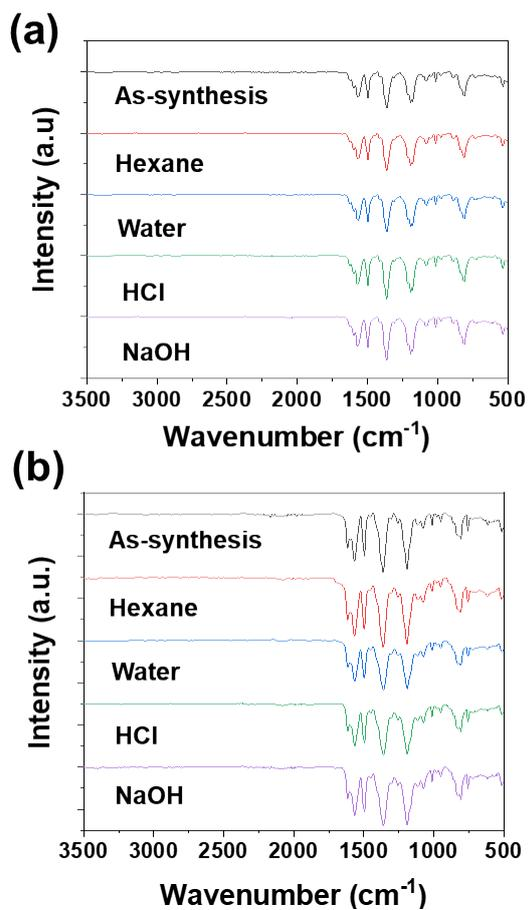
Fig. S7. FT IR spectra of (a) NI-COF-1 and (b) NI-COF-2 under different conditions.
