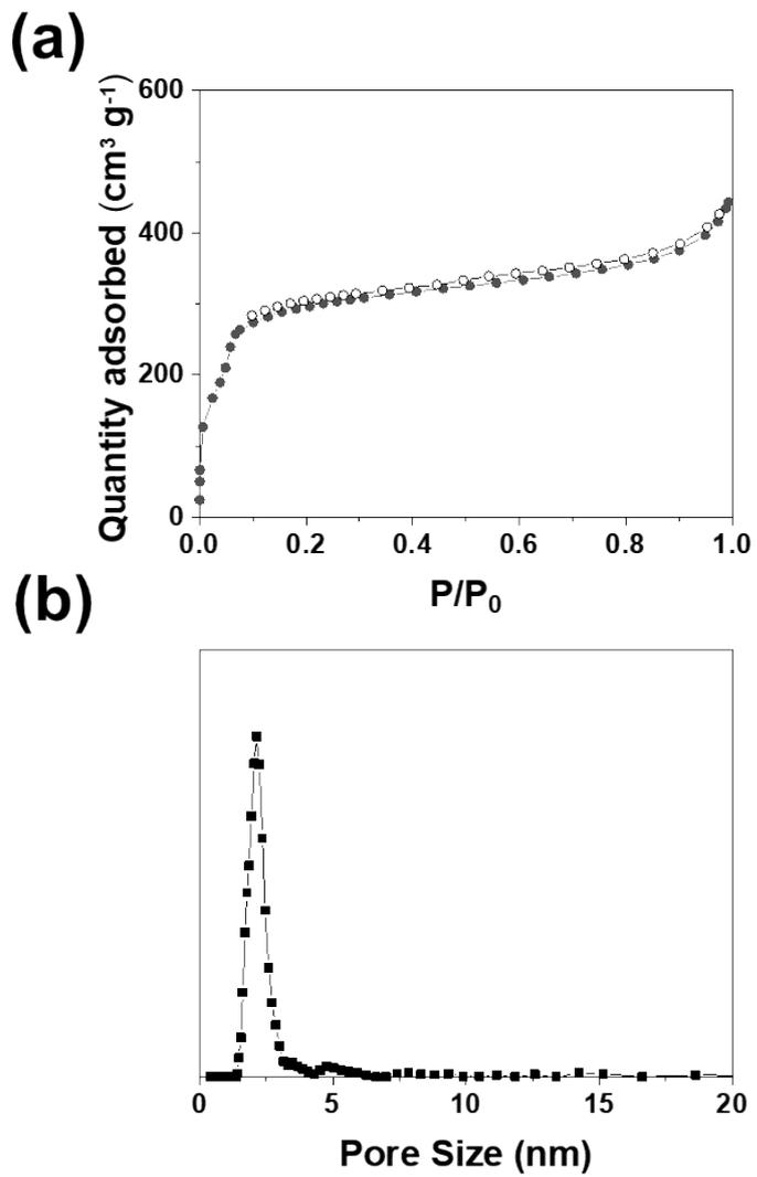
Fig. S6. Nitrogen adsorption-desorption isotherms of (a) NI-COF-2 measured at 77K (●: adsorption, ○: desorption). Pore size distribution of (b) NI-COF-2
