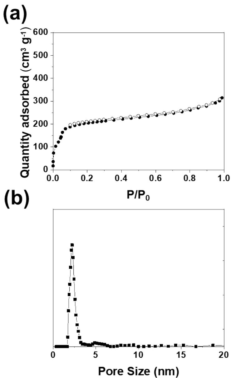
Fig. S5. Nitrogen adsorption-desorption isotherms of (a) NI-COF-1 measured at 77K (●: adsorption, ○: desorption). Pore size distribution of (b) NI-COF-1.
