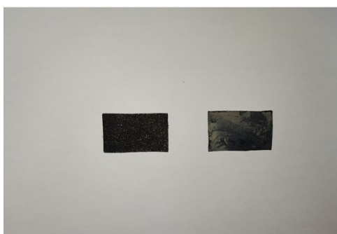
Fig. S1. Blank carbon cloth (left) and carbon cloth loaded with Zn/Co-3DHFLM (right).
