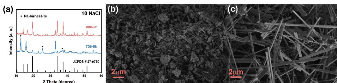
Figure S9. XRD patterns and SEM images of samples with NaCl molar ratio of 10 for 700-0h and 800-2h
