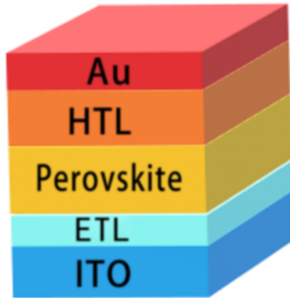
Fig. S1. Schematic device architecture of PSCs studied.
