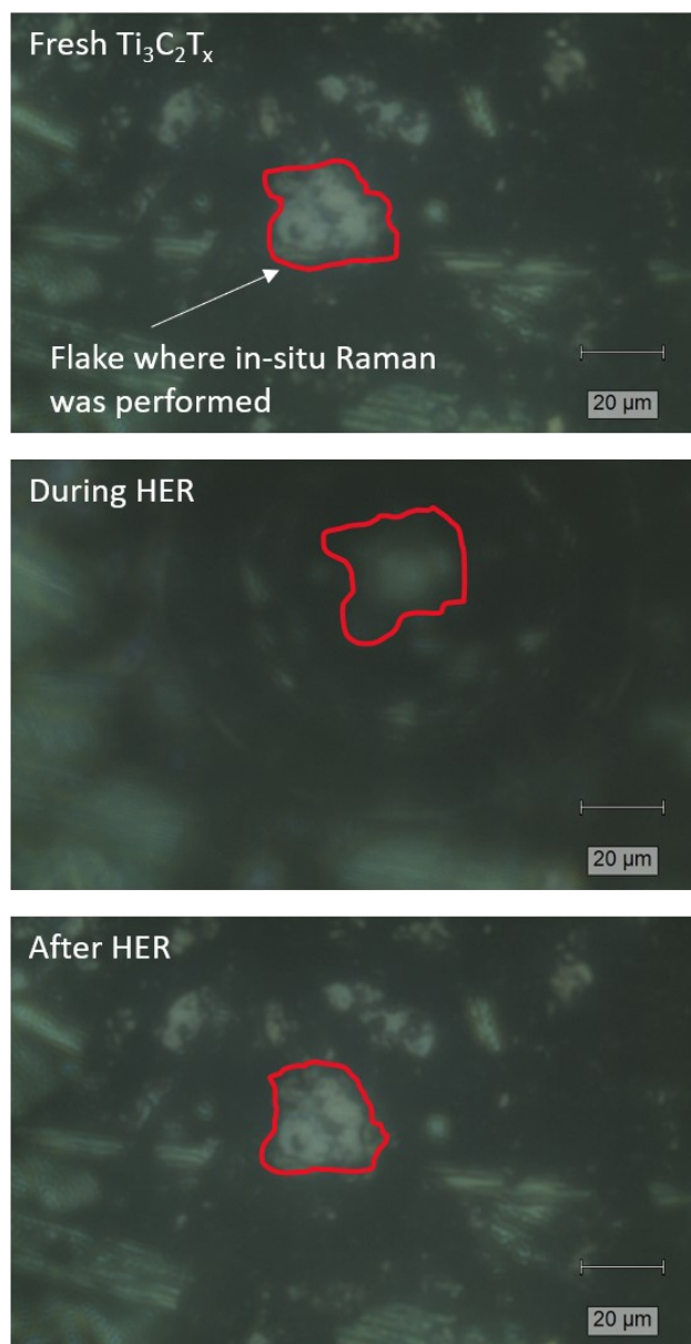
Figure S2. Images of \text{Ti}_3\text{C}_2\text{T}_x MXene flake before, during, and after HER process in acidic electrolyte as viewed through Raman eyepiece.
