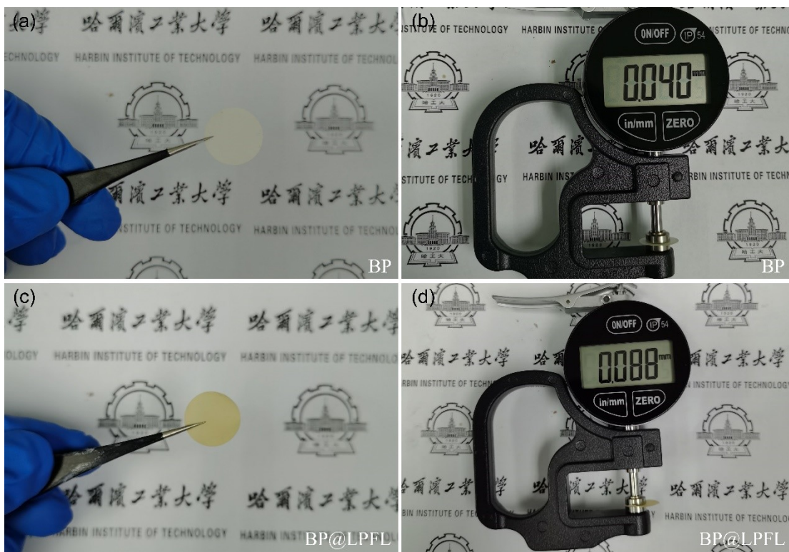
Fig. S4 (a) The digital photograph of the BP, (b) the thickness of BP film; (c) the digital photograph of the BP@LPFL, (d) the thickness of
