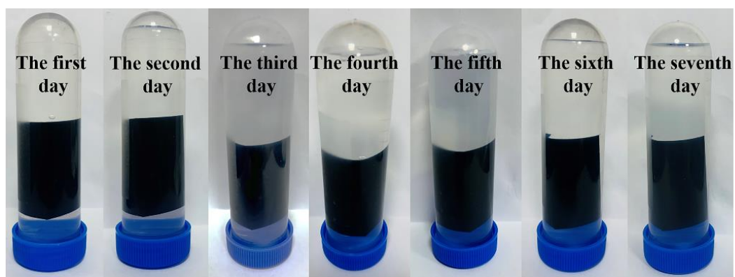
Figure S4. The digital photos of the PPy/filter paper soaked in water for 7 days.
