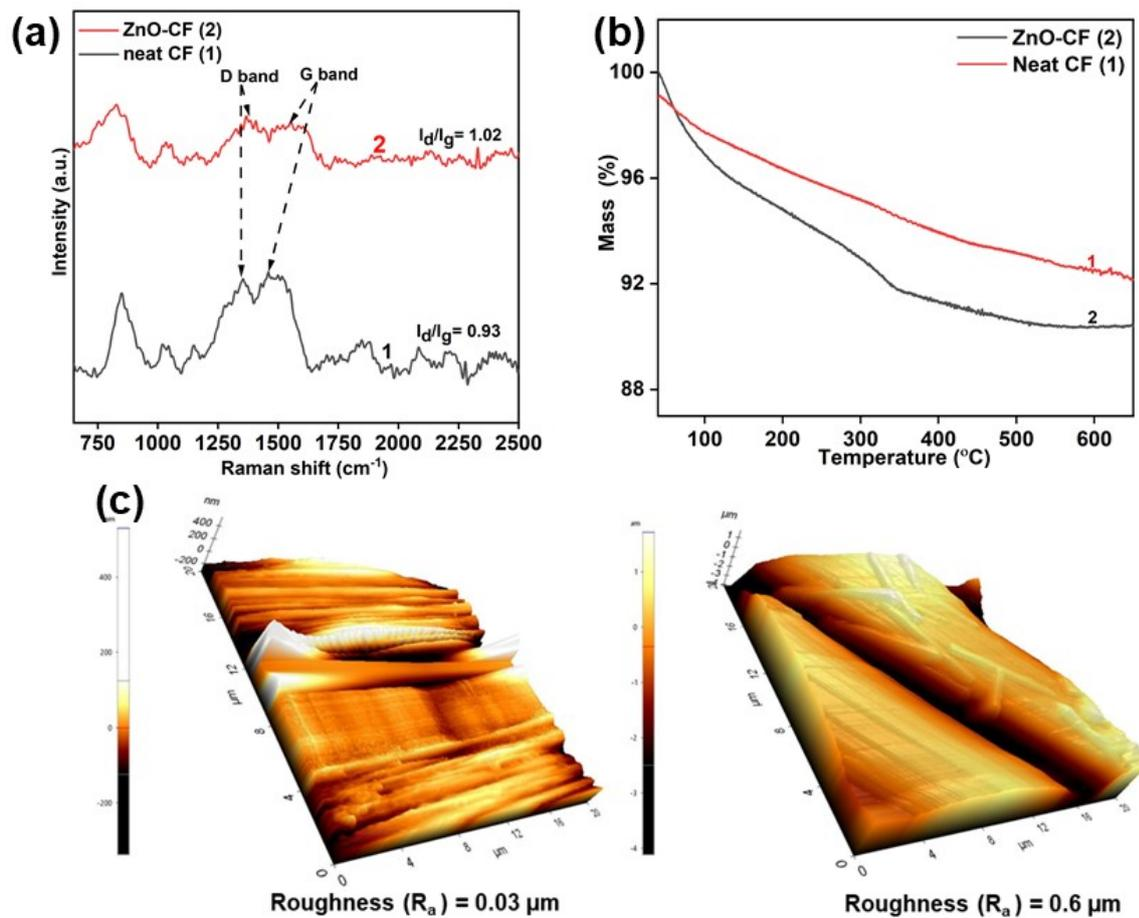
Figure S3: (a) Raman analysis (b) TGA analysis and (c) AFM analysis of neat CF and ZnO-CF
