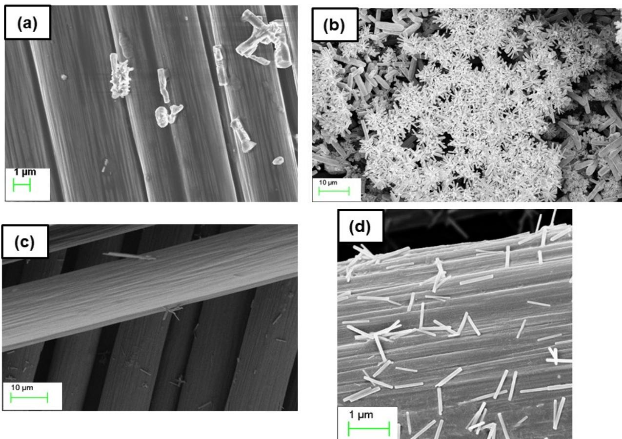
Figure S2: Growth of ZnO nano-rods on CF after (a) 5 min (b) 40 min and (C) 25 min of seed solution adsorption (d) Zoomed in image of (c) depicting the uniformity and distribution of ZnO nano-rods
