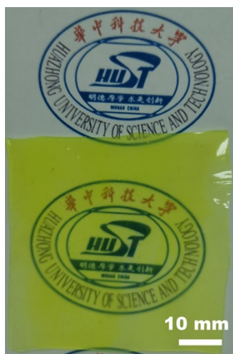
Figure S14. The quantum dot film on the pattern of Huazhong University of Science and Technology.
