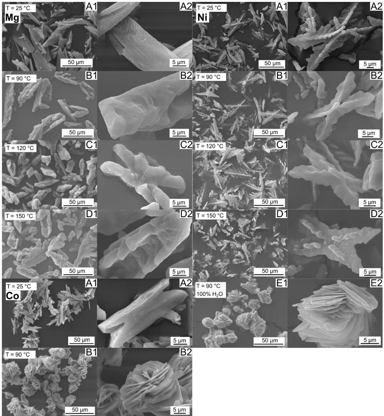
Figure S4: SE images of Mg-, Ni – and Co-struvite and their thermally-processed derivatives at given temperatures (90°C, 120°C, 150°C); an overview image at a low magnification, marked with 1 and a detailed view at an individual crystal, marked with 2; (A) M-struvite as synthesized at room temperature; (B) M-struvite isothermally-heated at T=90°C for t = 1 d; (C) Mg- and Ni-struvites isothermally-heated at T=120°C for t = 1 d; (D) Mg- and Ni-struvites isothermally-heated at T=150°C for t = 1 d; (E) Ni-struvite isothermally heated for t = 1 d in a 100% H 2 O environment (hydrothermal synthesis). While amorphous Ni-containing phosphates mimic the relict crystalline Ni-struvite morphology, except the hydrothermal sample, the Co-phosphates change their crystalline habit due to multiple crystalline phase transitions.
