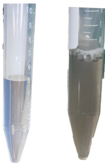
Figure S4. Gas bubbles observed after incubation of 1.0 mM \text{H}_2\text{O}_2 with phosphate buffered solution (0.1 M, pH = 6.2) (Left) and BSA@ \text{Gd}_2\text{O}_3/\text{IrO}_2 NPs (Ir equivalent concentration: 2.0 mM) (Right) for 5 min.
