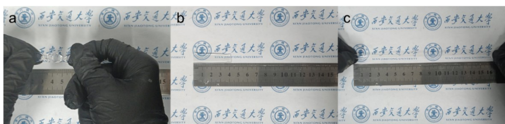
Figure S20. The mechanical flexibility test of quasi-solid-state gel. Twisting (a), and stretching (b-c).
