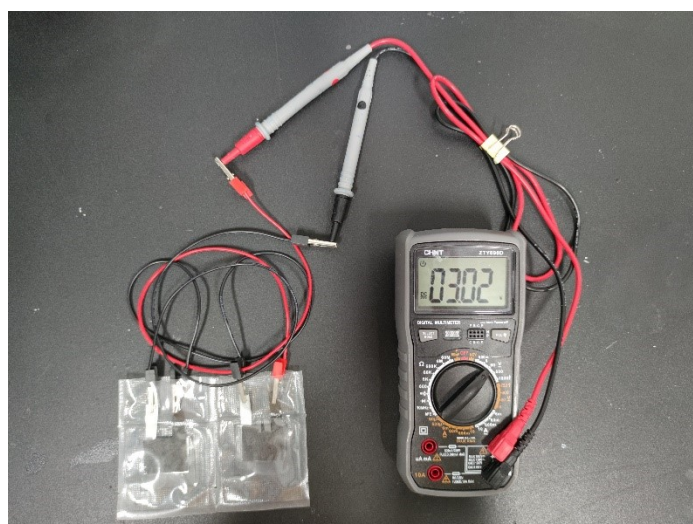
Figure S24. The open voltage of two quasi-solid-state cells linked in series.
