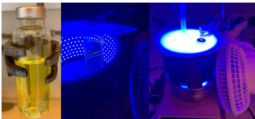
Figure S2. Scale-up experiment for the hydroacylation of 2a : microwave vial (left), and the reaction setup (middle and right).
