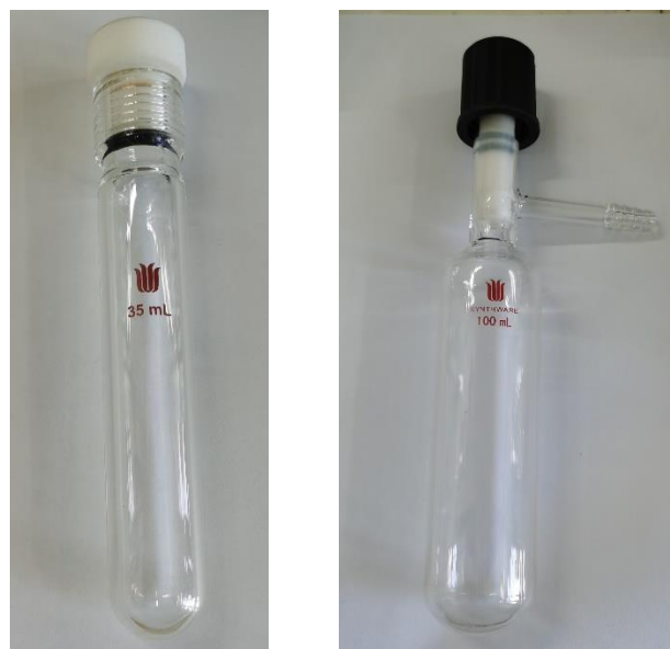
Figure S1. Pressure sealed tubes for reactions
