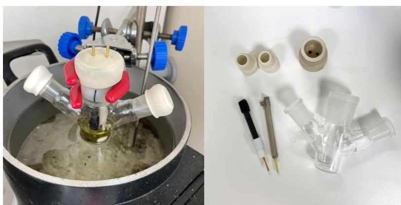
Figure S1. The electrolysis setup [The RVC is fixed on a sharpened graphite rod ( \varnothing 6 mm)].
