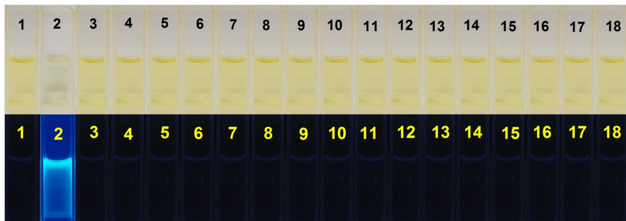
Fig. S7. Photograph of colorimetric changes (upper panel) and fluorescence responses (lower panel) of NAN (1 \mu M) to various bio-relevant cations [From left to right: 1) Only NAN, NAN with 2) Al 3+ 3) Sn 2+ , 4) Zn 2+ , 5) Cu 2+ , 6) Hg 2+ , 7) Cd 2+ , 8) Mg 2+ , 9) Pb 2+ , 10) Fe 2+ , 11) Fe 3+ , 12)
