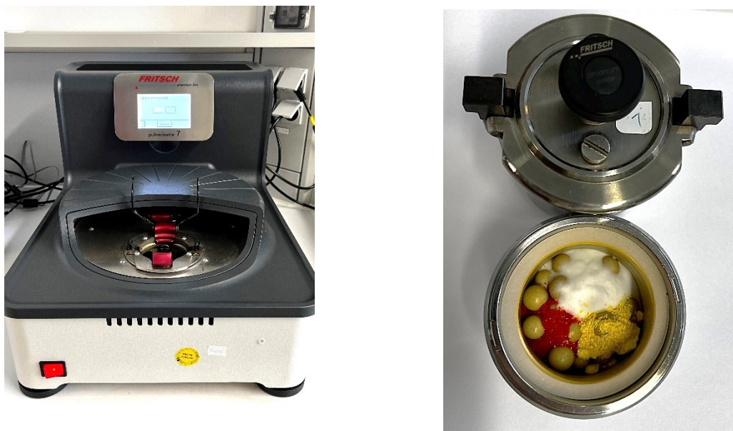
Figure F1: Pulverisette 7 Premium Line with the respective milling jars.
