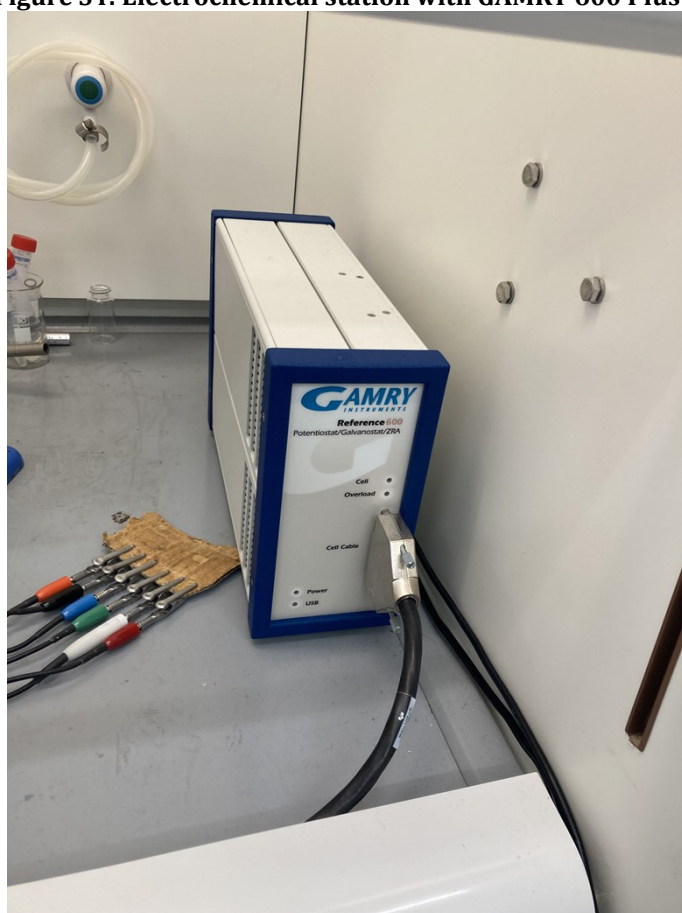
Figure S5: Electrochemical station with GAMRY 600 potentiostat
