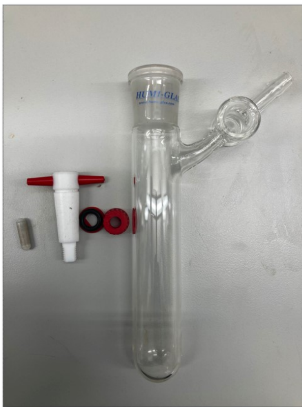
Figure S1: Glassware setup for electrochemical reactions
