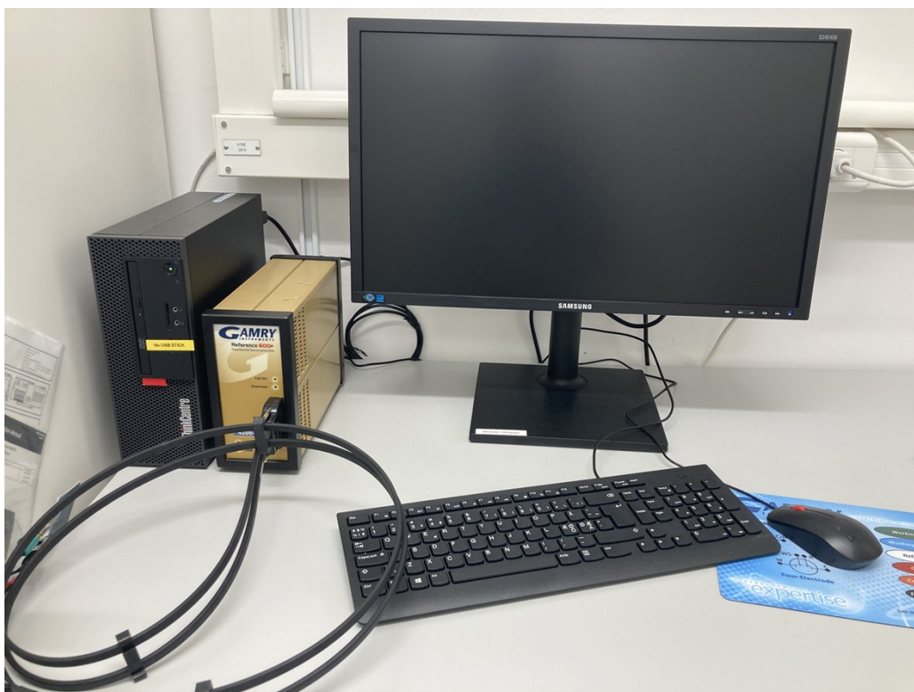
Figure S4: Electrochemical station with GAMRY 600 Plus potentiostat
