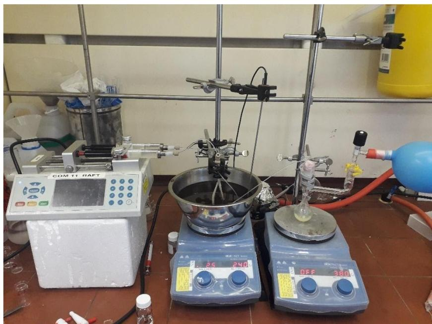
**Figure S3.** Picture of the setup for the continuous flow organocatalysed polymerisation and post-modification reactions.
